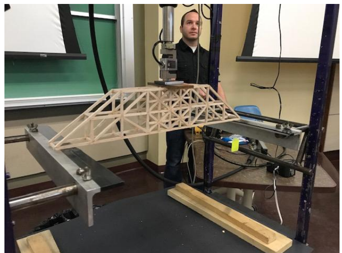
Bridge models testing in progress
