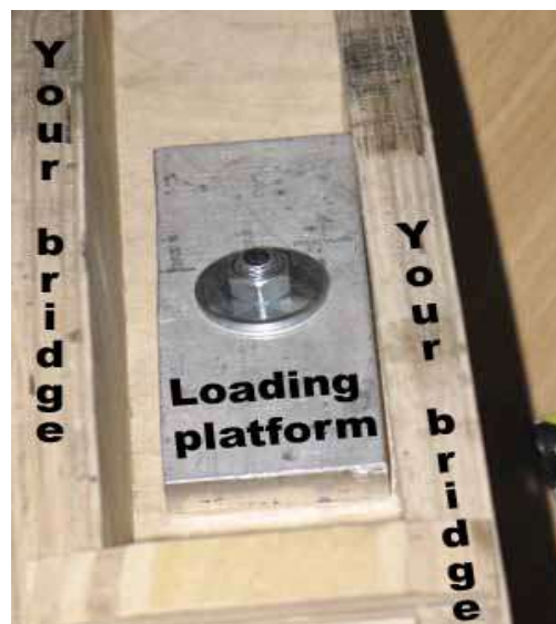
Picture 3: Loading Platform attached to a bridge
